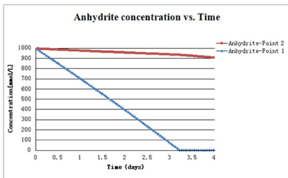
Fig.2: Anhydrite concentrations as a function of time at observation point 1 and 2
