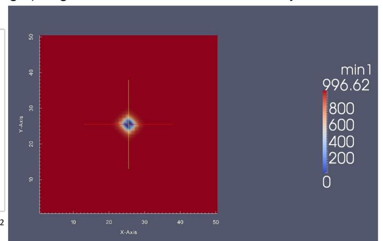
Fig.4: Anhydrite distribution after 4 days. The amount of anhydrite is reduced to zero in a radius of about 3 m around the well (unit is mmol/L).
