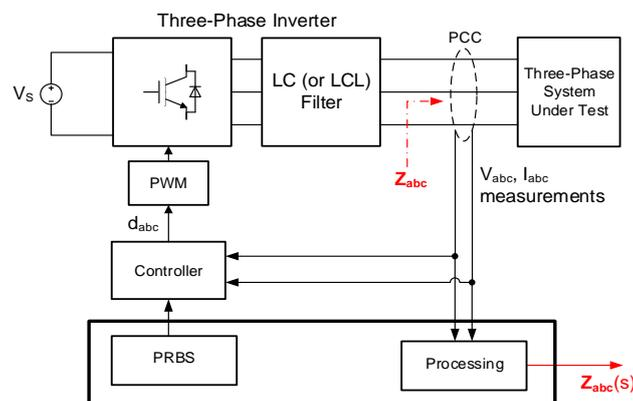
Figure 1: block diagram of the WSI technique for for online parametric identification of AC Power Grid Impedances.
