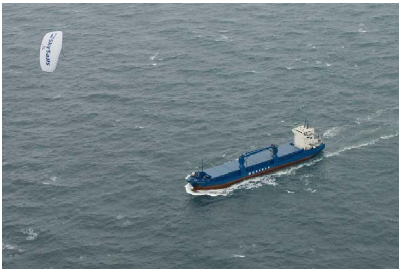
Fig. 4. SkySails system installed on freight vessel “MV Michael A.”
