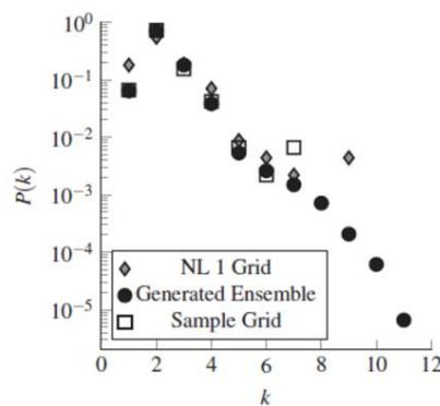
**Figure 2** Intuitive illustration of the 'statistical similarity' concept between one real distribution grid (in the figure, "NL1 Grid") and a set of generated test grids (in the figure, "Generated Ensemble"). As it can be seen, the real grid (diamonds) and the set of generated test grids (filled circles) exhibit the same statistical distribution of  $P(k)$ , a basic CN metrics [2]
